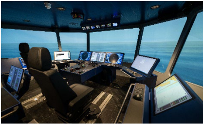
The 16 m wide Full Mission Bridge (FMB) with cylindrical projection forward/backward and domes of 6 m wide at both bridge wings to allow forward, backward, downward and upward views during port and other complex operations.
