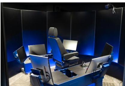
Multi-Purpose Simulator (MPS) with 360 degrees projection for coupled tug or crane simulations.
